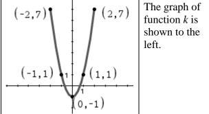
Use the given coordinates to calculate the rates of change as the input values increase. What do you notice about the rates of change and what can you say about the concavity of the graph of the function based on the rates of change? Rates of change over equal length input-value intervals: -6, -2, 2, 6. The rates of change increase so the function is concave up on the interval (-2,2). EK: 1.1.B.3
